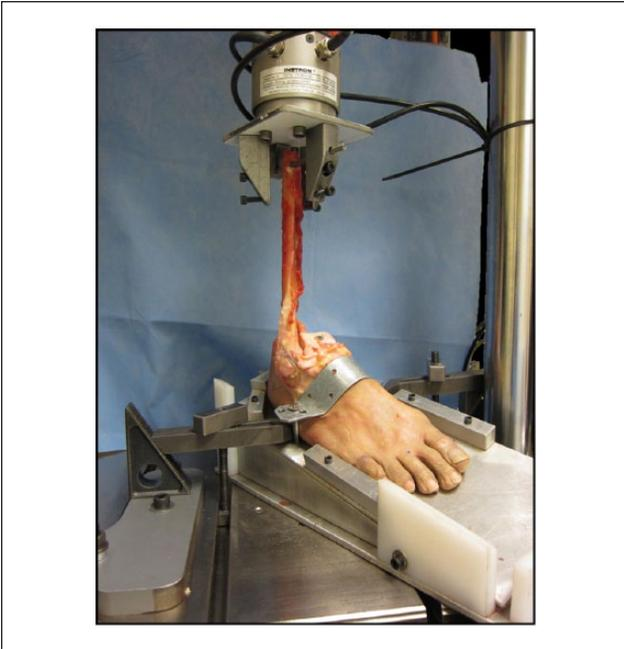
**Figure 3.** Right foot and ankle specimen secured to the load actuator of the dynamic tensile testing machine via a 6-mm-diameter pin placed lateral to medial through a reamed fibular tunnel. The specimen was secured to the base via a custom jig that positioned the specimen in 20 degrees of inversion and 10 degrees of plantarflexion relative to the vertical fibula.
