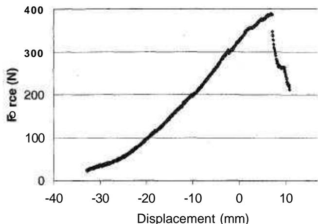
Fig. 2: Load displacement curve for tendon to tendon fixation.
