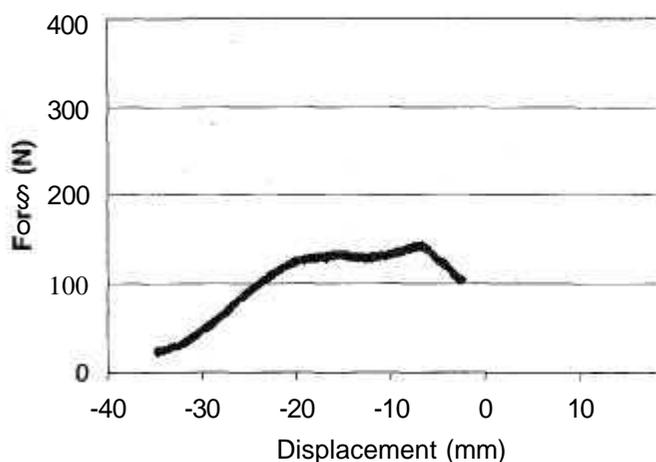
Fig. 3: Load displacement curve for bioabsorbable screw fixation.
