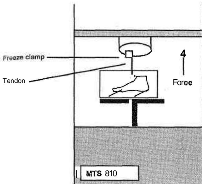
Fig. 1: The tendon is attached to the testing ram of the material testing system through a freeze clamp. The cadaver specimen is anchored to the system base through smooth wires placed in the calcaneus and first metatarsal.
